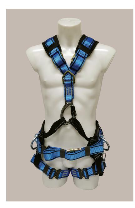
Yoke harness designed for use on wood poles and transmission towers. Heavy wearing polyester webbing for enhanced durability, sliding side D rings and ergonomic wait pad for added comfort and durability. Fully openable to allow easy donning and doffing, it is designed to be comfortable to wear all day and not restrict movement while moving or climbing.
