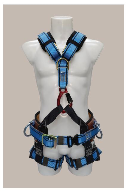
Yoke harness designed for use on wood poles and transmission towers. Heavy wearing polyester webbing for enhanced durability, sliding side D rings and leather wait pad for added comfort and durability. Fully openable to allow easy donning and doffing, it is designed to be comfortable to wear all day and not restrict movement while moving or climbing.
