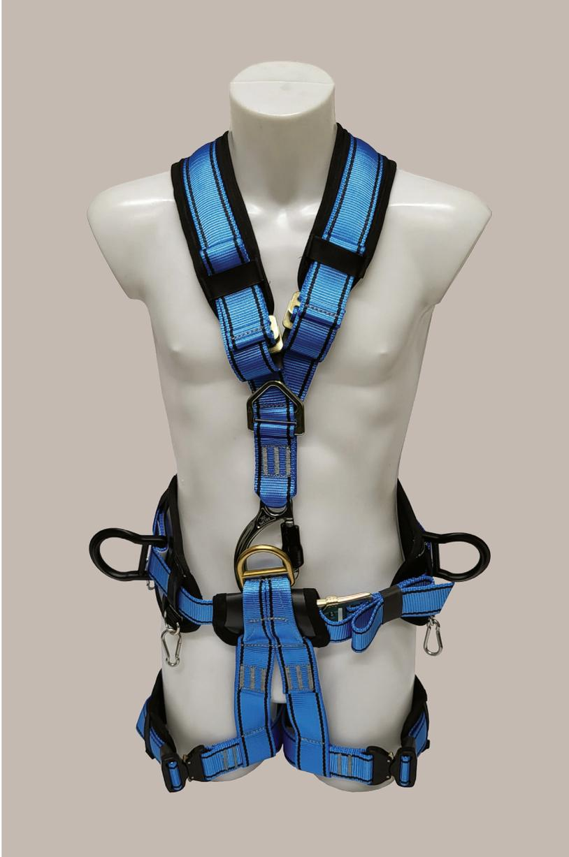
Yoke harness designed for use on wood poles and transmission towers. Heavy wearing polyester webbing for enhanced durability, sliding side D rings and ergonomic waist pad for added comfort. Certified as a full bodied sit harness, it is designed to be comfortable to wear all day and not restrict movement while moving or climbing.
