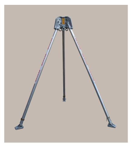
The RT3 has 6 anchor points, each tested to EN795. The 3 overhead pulleys hold up to 11mm rope and the extra swivel anchor points may be used with pulleys for a double roped rescuer, back-up system, airlines, communication lines, medical kits, tools etc.
