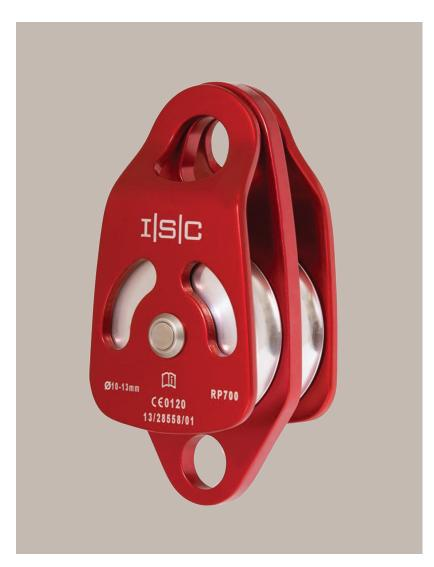
One way locking bearings are ideal for lifting & lowering applications. The wheel locks is one direction to provide maximum friction, which allows for greater control while lowering. When operated in the opposite direction, the wheel is free-running to reduce friction to a minimum, for greater ease of use when lifting.
