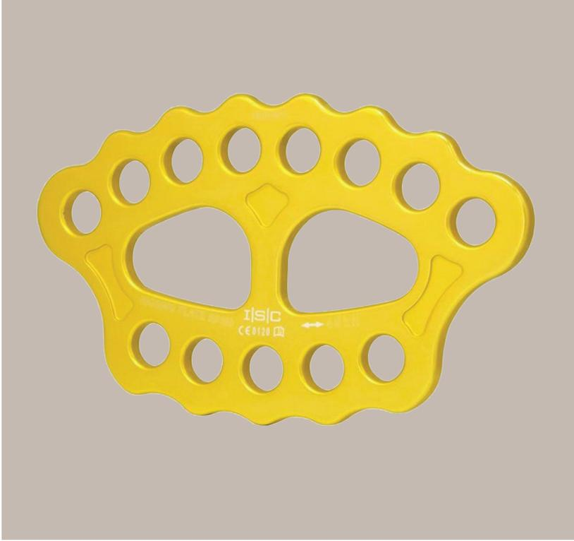
Rigging Plates are made from high strength aluminium and have 20mm (over 3/4") holes, to allow Karabiners to be fully rotated.
