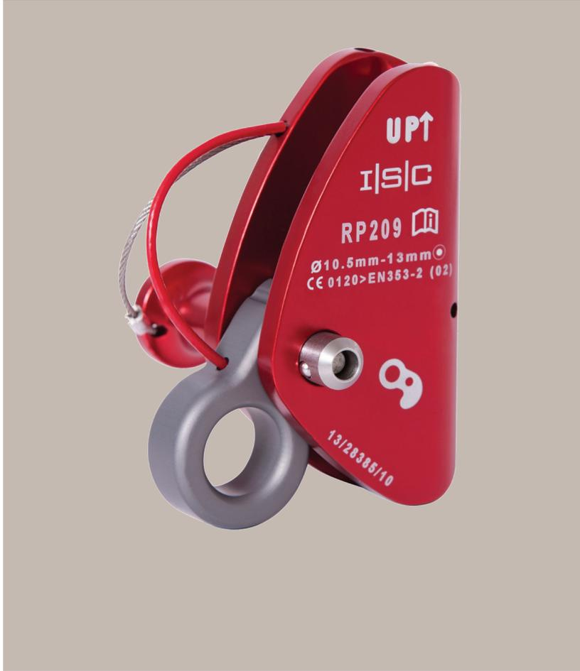
The RP209 Ropegrab has a pip pin axle, allowing the Ropegrab to easily be fitted or removed from the working rope line at anytime, without the need for the user to detach from their harness.
