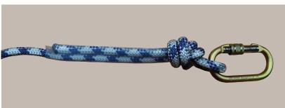
32 strand Polyamide construction provides excellent wear resistance, good grip and lovely handling characteristics.
