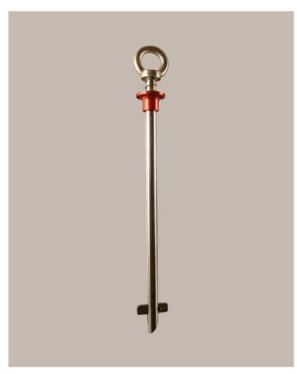
Girder & Concrete Anchors are a quick and easy portable anchorage solution and can be used in the vertical and horizontal plane. These anchors are operated by using two fingers to pull back the red collar. This action retracts the retention bar, allowing the device to be inserted into the anchor hole. Once the device is in position, the red collar can be release, causing the retention bar to engage, fixing the device in position.
