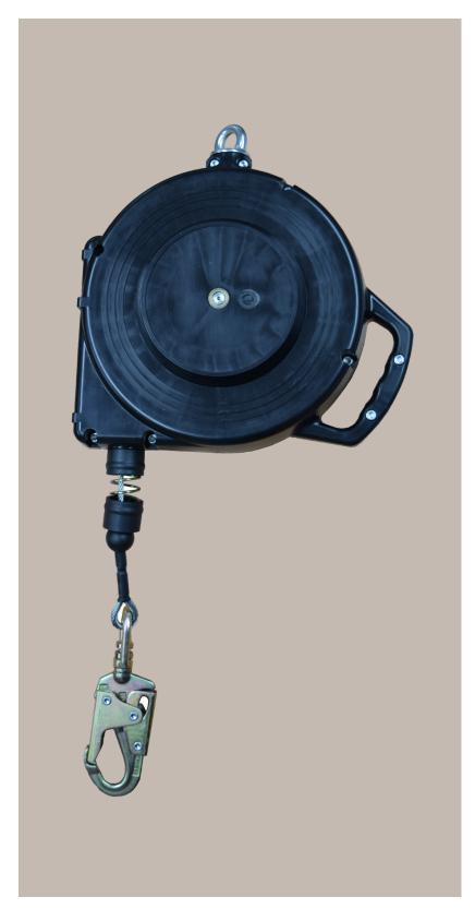
The 30m Fall Arrest Device is designed to provide fall protection from falls from height. Anchored above the user, it gives the user a safe area of work. The retracting line pays in and out of the device as the user moves. In the event of a fall, a brake engages, arresting the fall of the user with a controlled deceleration force.
