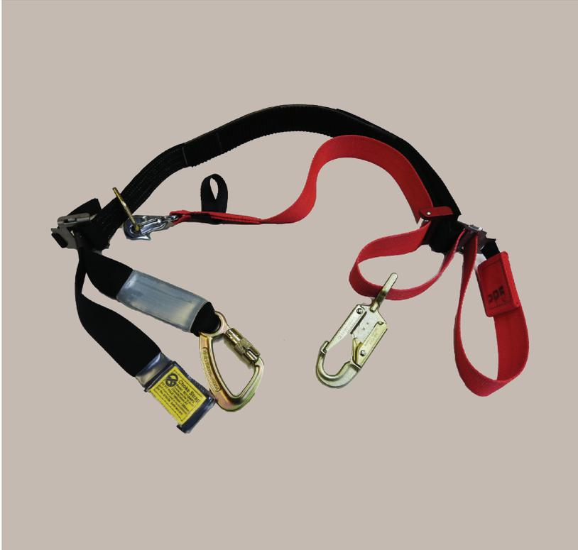
The Choke Strap is designed for use by electrical utility personnel for ascending and descending wood poles and will arrest the wearer in case of a fall, the choke strap can also be used as a work positioning belt if used in conjunction with a secondary fall arrest device. It was designed to be used by left or right handed people and is fully adjustable for use on a range of different sized wood poles with a smaller version being available for small diameter poles.
