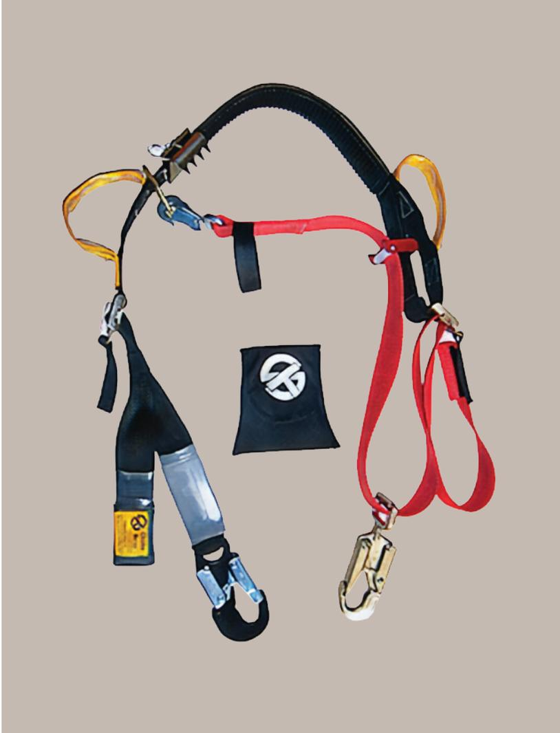
The Choke Strap is designed for use by electrical utility personnel for ascending and descending wood poles and will arrest the wearer in case of a fall, the choke strap can also be used as a work positioning belt if used in conjunction with a secondary fall arrest device. It was designed to be used by left or right handed people and is fully adjustable for use on a range of different sized wood poles with a smaller version being available for small diameter poles.
