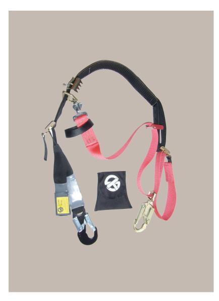
The Choke Strap has been designed for use by electrical utility personnel for ascending and descending wood poles and will arrest the wearer in case of a fall. It can also be used as a work positioning belt if used in conjunction with a secondary fall arrest device.
