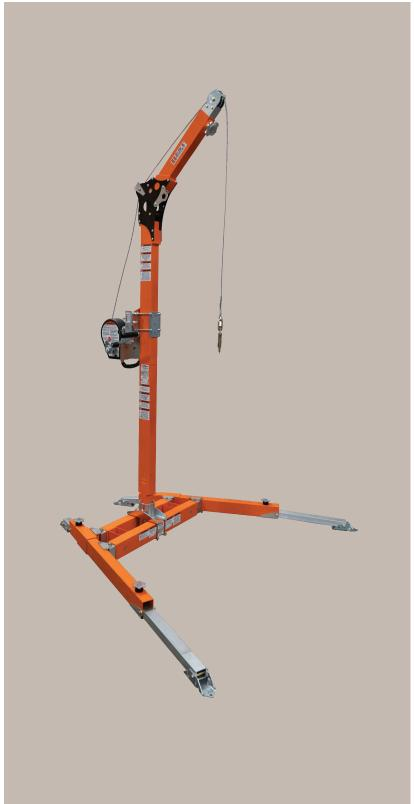
The 30070 portable base has four independent support legs. The main support legs can also be adjusted outward, so the base can "wrapped" around a hole with a 54" to 75" diameter. The davit sleeve may also be moved left to right to allow rotating the davit in rescue applications.
