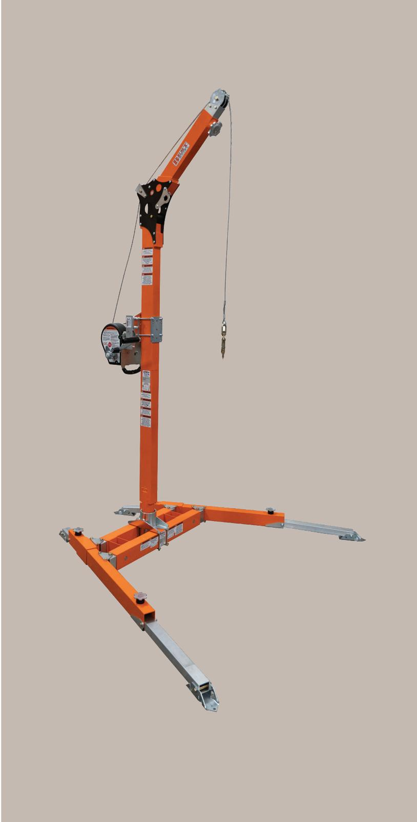
The 30070 portable base has four independent support legs. The main support legs can also be adjusted outward, so the base can “wrapped” around a hole with a 54” to 75” diameter. The davit sleeve may also be moved left to right to allow rotating the davit in rescue applications.
