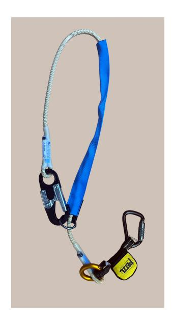
Lightweight 1.75m fall arrest lanyard featuring a heat- and cut-resistant Technora® braid rope, designed for enhanced safety in extreme environments.
